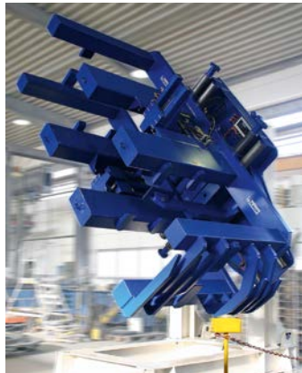
25T251W/099 - Inverter for steel sheets
